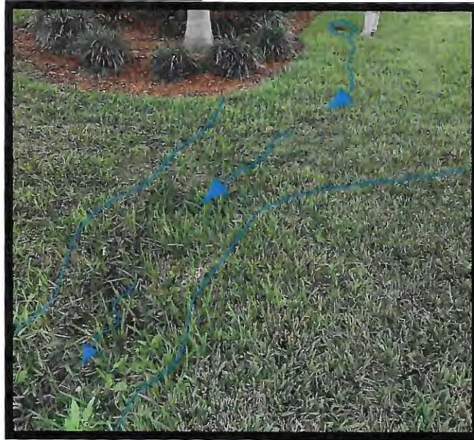
Figure 3: Evidence of sheet flow channeling to lake (Northwest property line)
